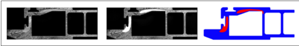
Figure 2-6 Image processing of samples. Left: photographically recorded cross-section, centre: marking of the transition, right: final processed contour.
