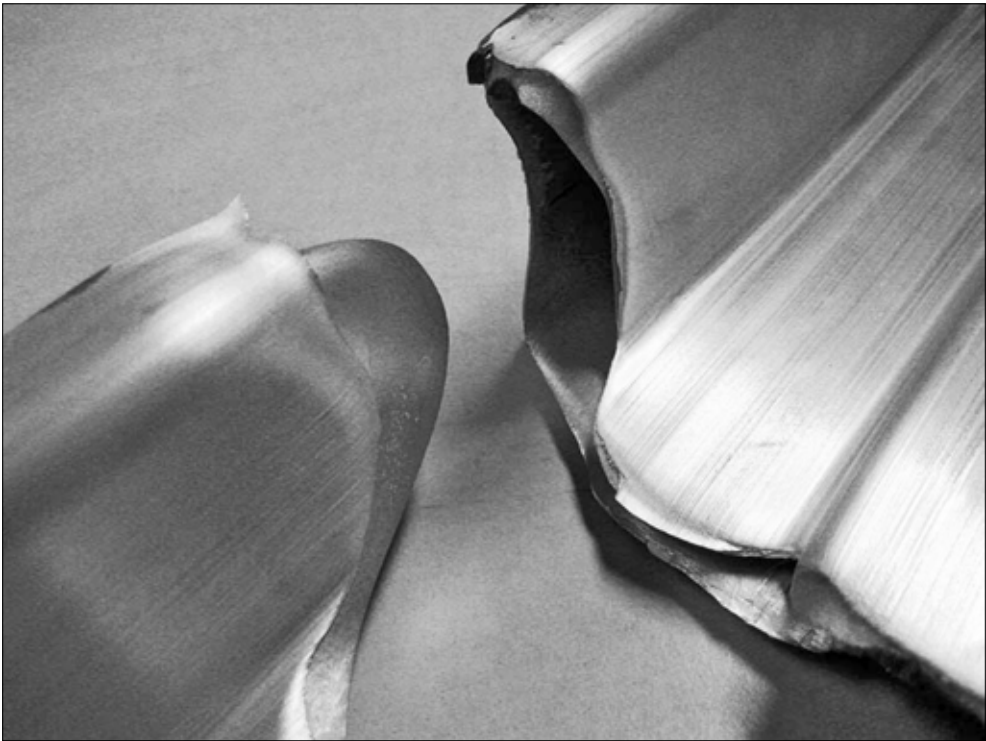
Figure 1-1 Detail of an extrusion separated at the charge weld interface, revealing the bulbous cusp of new material and shear lips at the peripheral, well bonded areas.
